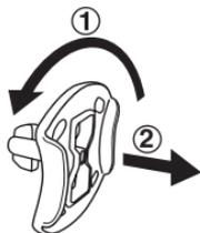
① Rotate the packaging locks 90 degrees anticlockwise.
